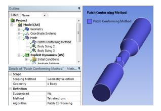
Insert a Mesh Sizing using Type, Sphere of Influence. For Sphere Center, select the previously created Coordinate System. Insert these values.
