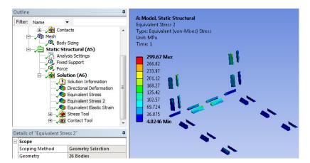
Contact Tool only in the Frictional Contacts, as seen here.
