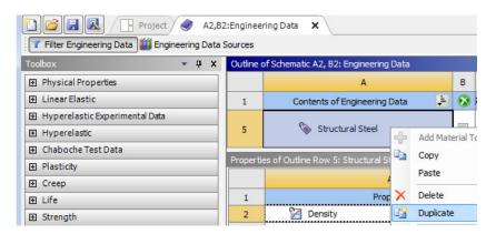
Suppress the fields shown here with strikethrough font by checking them in column D. Name the material as POM.
