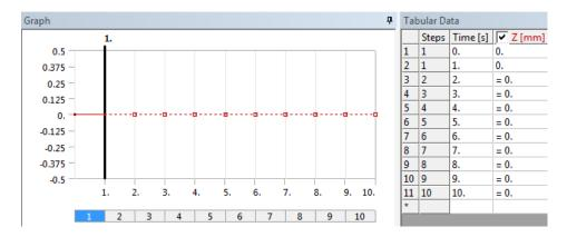
Insert a Displacement by selecting all the outer faces, green here, of the Die, except the ones inside, where the Sheet will be bent and touch the Die, Apply. Make sure that you have selected 5 faces.
