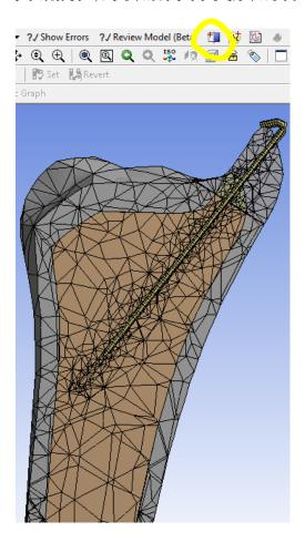
Static Structural, Analysis Settings: Make Number Of Steps = 3 then insert these details for each step.
