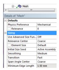
On the Punch and Die, blue here, apply a Mesh Sizing
