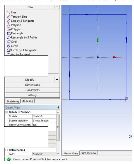
Got to the Modeling tab. There is no need to Extrude a sketch if it is shown with green check symbol. Press the Extrude button. Observe
