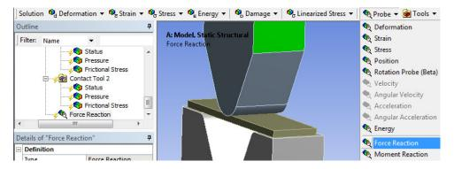
Make Boundary Condition = Displacement (the one we created on the punch). Solve.
