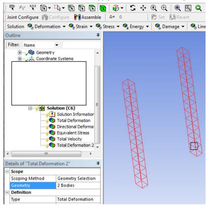
Insert an Equivalent Stress only on the Line Bodies (red here). Solve.
